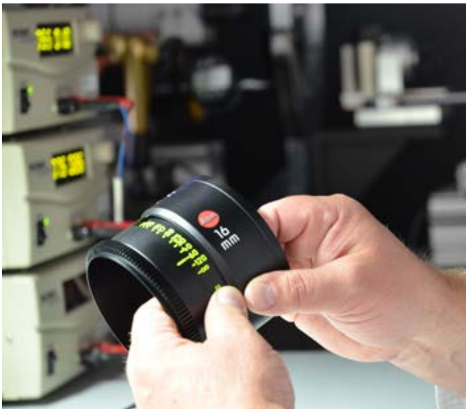
Assembly begins: the mechanical focus components are prepared prior to installing the optical elements
