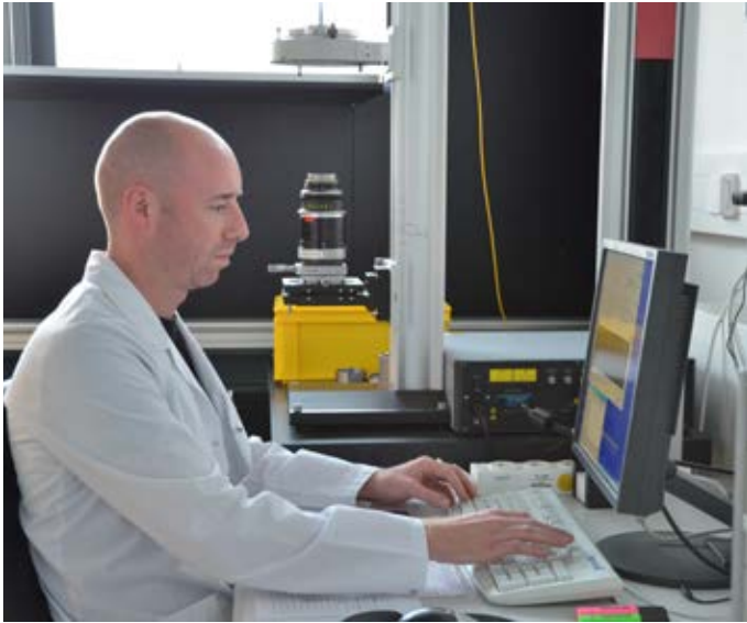
Measuring air gaps of completed lens
