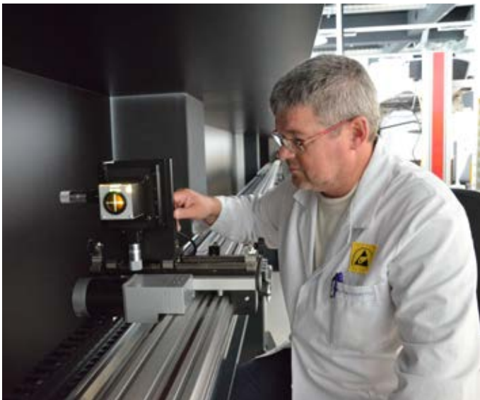
The target is controlled from the computer, moving to the pre-determined distance for each focus mark calibration.
