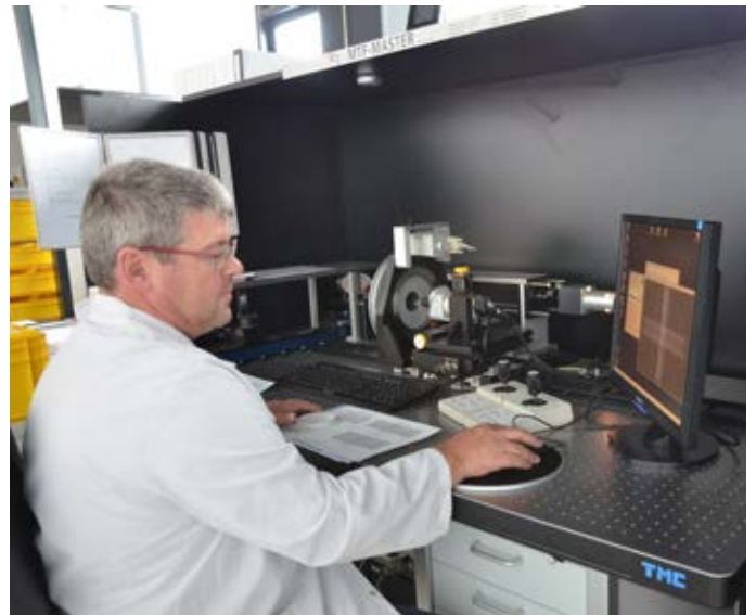
Racking lens focus remotely while looking at a computer read-out of MTF contrast. When the optimum setting is achieved, he clicks "save," and the setting is stored. The data goes to a laser engraving machine. Each focus ring is therefore optimized for each lens.
