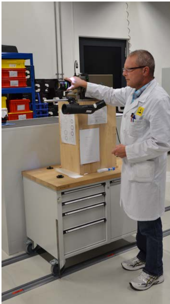
Lenses are checked on the lens projector at several intervals during the assembly process.
