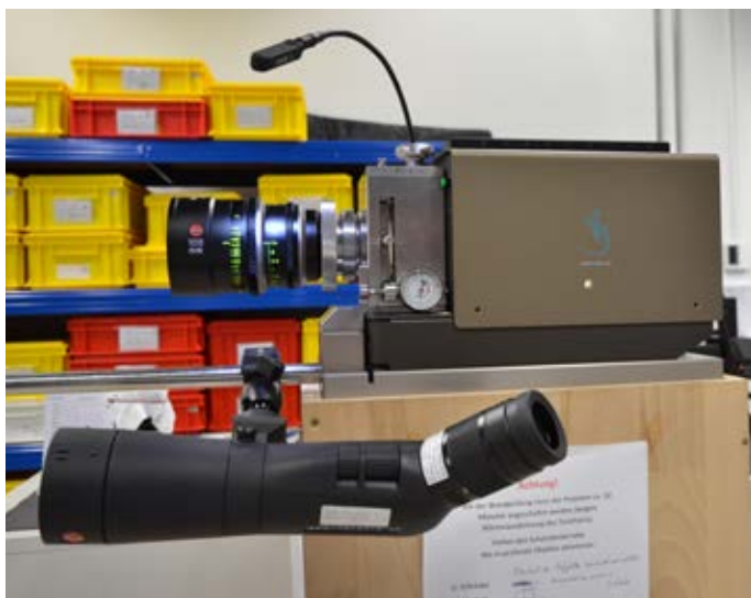
Familiar lens projection tools: a Gecko-Cam lens projector and Leica APO-Televid 65 spotting scope to check image sharpness.
