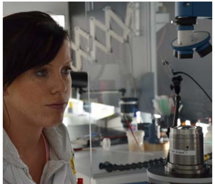
Checking optical centering
